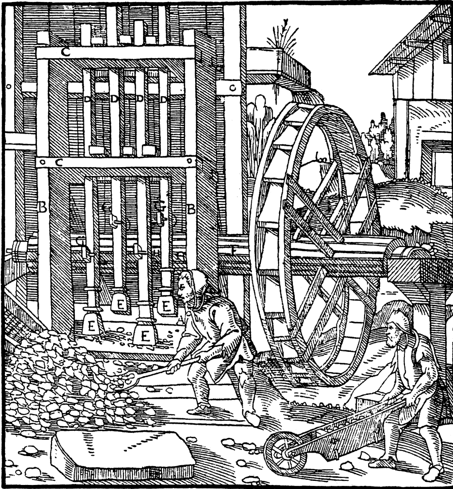
FIG. 4. MEDIEVAL ORE-CRUSHING MACHINE ILLUSTRATED IN AGRICOLA'S DE RE METALLICA (BOOK 8). AN OVERSHOT WATER-WHEEL TURNS AN AXLE ON WHICH CAMS RAISE AND DROP STAMPS SHOD WITH METAL HEADS (E) TO CRUSH ORE SHOVELLED ONTO THE ANVIL BENEATH THEM. THE STONES ILLUSTRATED IN FIG. 3 ARE ANVILS BELONGING TO A SIMILAR KIND OF MACHINE. (Georgius Agricola, De Re Metallica , translated by H. C. Hoover and L. H. Hoover (Dover Publications Inc. 1950), 284)
